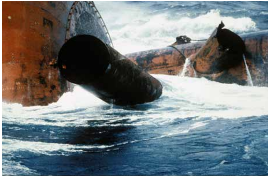
Photo: Unknown / ConocoPhillips / Norwegian Petroleum Museum The broken D-column floating in the sea.
