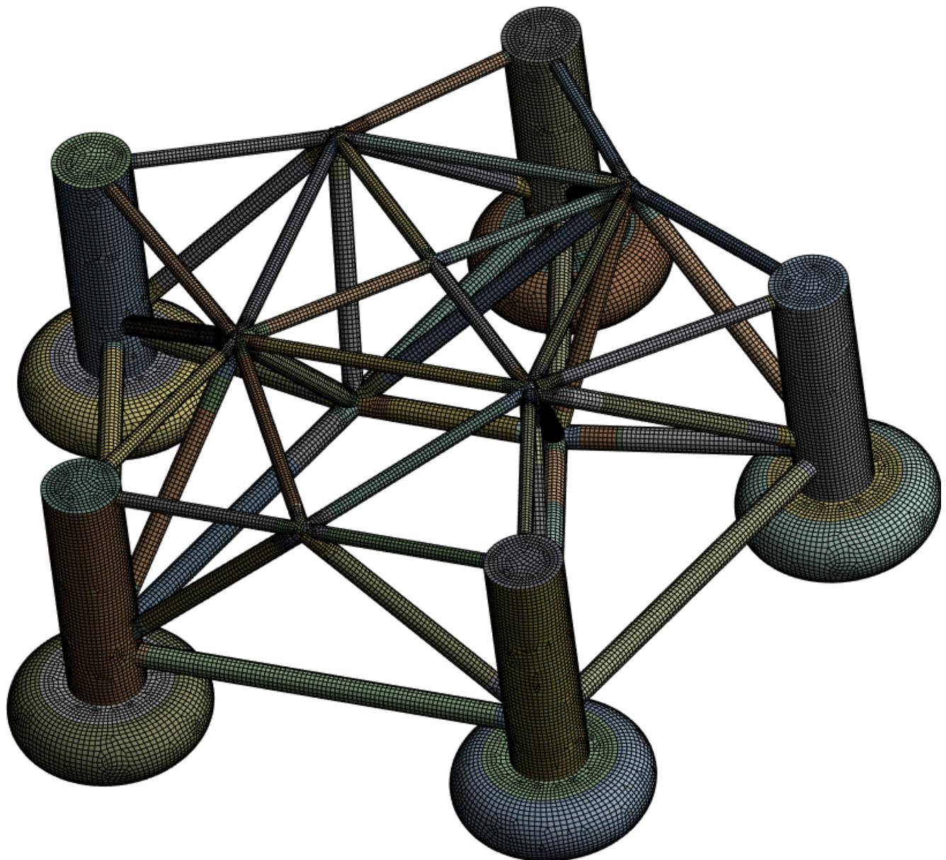
The figure below show the applied load of 3080 kN equally divided on the 5 columns, 616 kN on each.
