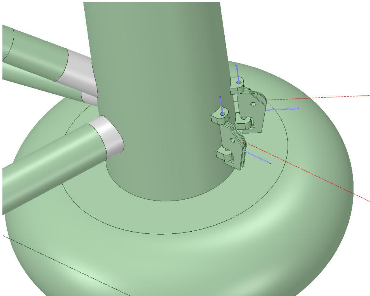
The figure below show the fairled orientation at D-leg for the two anchoring patterns. Note that for the ideal 10 line configuration the anchor forces do not give additional torque in the main column.
