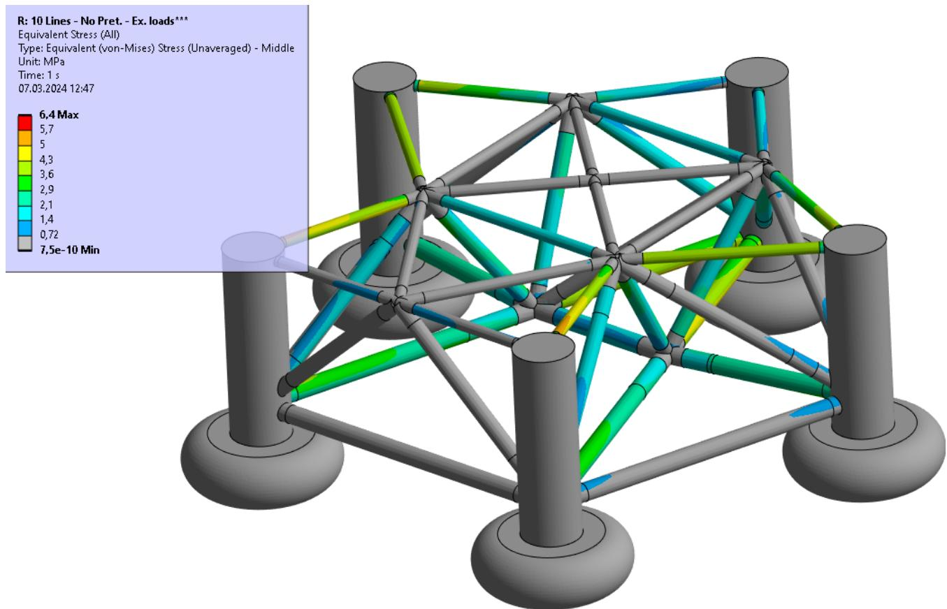
The following plot shows the Equivalent (von-Mises) stress for the 8 line un-symmetric pattern on Edda 2/7C.
