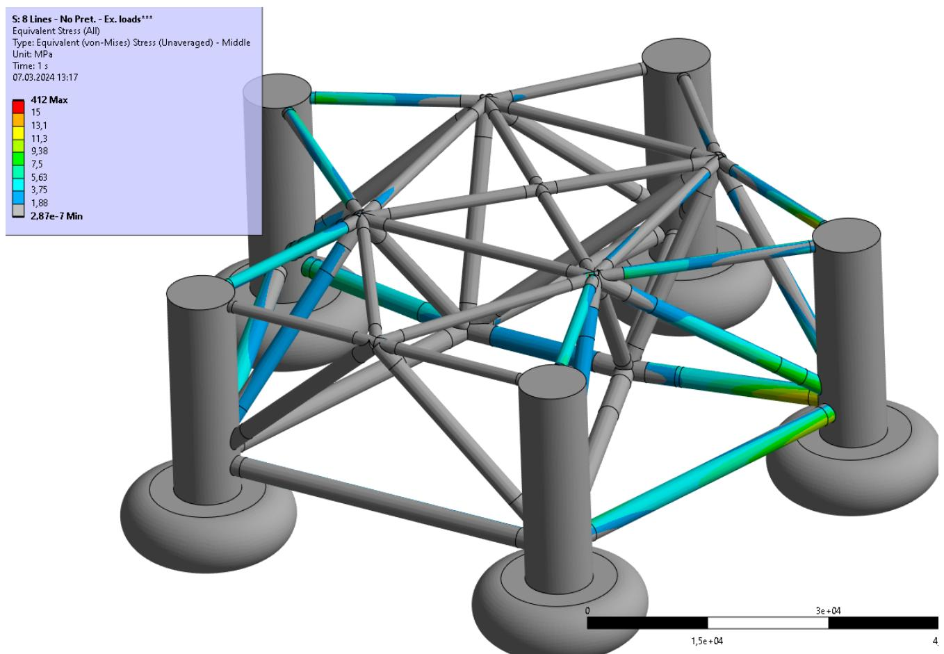
Note that some high peak stresses occur in the stiff joints (1-7) which is due to the simplified model of these joints combined with some elements with poor quality in this area.
